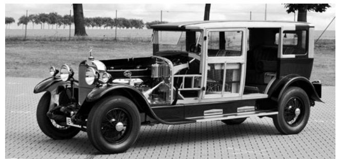
1925 Cutaway model of the Audi 18/70 PS Type M: The wooden chassis can clearly be seen (© Audi)
