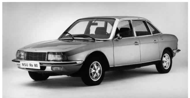
1967 Works photo of the NSU Ro 80: The pioneering design resulted in a drag coefficient of 0.37 (© Audi)
