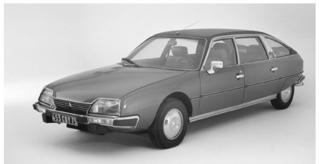
1974 In the case of the Citroën CX the drag coefficient is part of the model name, because c_x is the French abbreviation used for the measurement (© Citroën)
